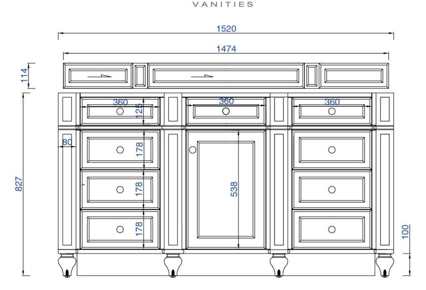
NOTE ONE: Countertops are not shown in these diagrams. (Cabinet Only) NOTE TWO: Wood Backsplash (Shown) is designed for the molding detail to align with sinks in James Martin's Optional Countertops.
